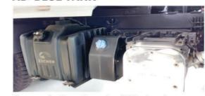
Urea section from the tank to UDS takes place through pick-up filter by vibrating diaphragm pump. Urea is then pressurized to injection line & pushed towards nozzle.
